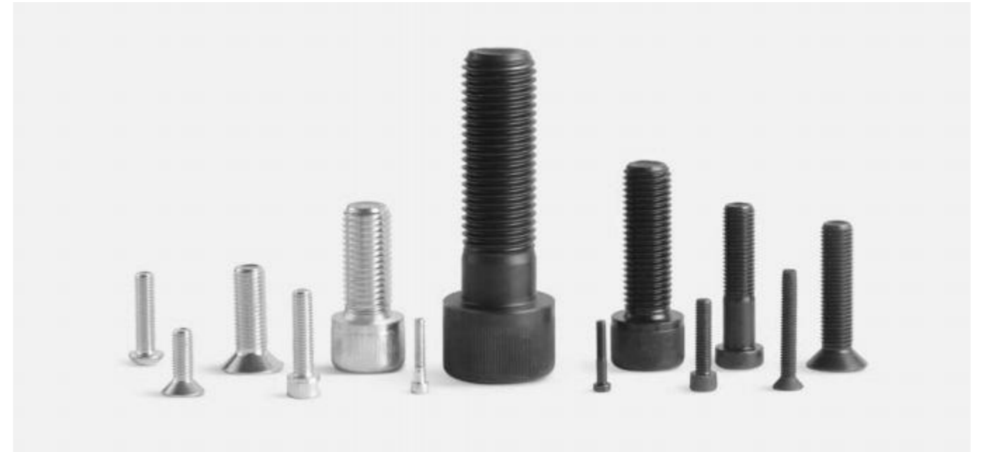
Hexagon Socket Head Cap Screws, Hexagon Socket Head Cap Screws with Low Head, Hexagon Socket Countersunk Head Screws, Hexagon Socket Button Head Screws Standard: DIN912 / DIN7984 / DIN7991, ISO4762 / ISO10642 / ISO7380-1, ASME B18.3 Grade: 8.8 / 10.9 / 12.9, 08.8 / 010.9, A574 / F835 Diameter: M3 - M42 (8# - 2")
