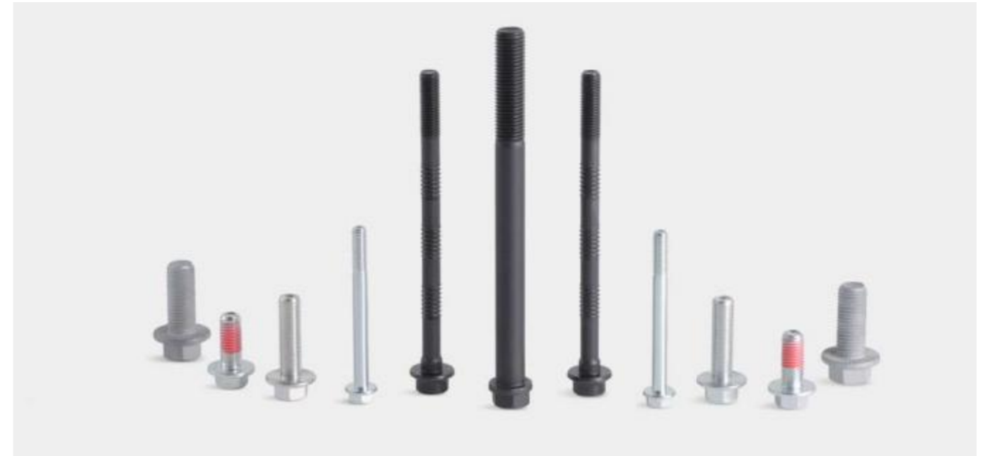
Hex Flange Bolts Standard: IFI-111 / DIN6921 / EN1665 / ISO4162 / JIS B1189 Grade: 5 / 8, 8.8 / 10.9 / 12.9, CL-90 / CL-100 Diameter: 1/4" - 3/4" (M5 - M20)
